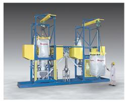
Bulk Bag Weigh Batch Eductor System features dual bulk bag unloaders, each with integral bulk bag conditioners and flexible screw conveyors feeding a central eductor that feeds solid material into a liquid stream.
